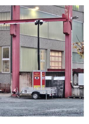
All are mounted on a mobile tower and offer 360-degree, 24/7 monitoring with a detection range of 400 meters during the day and 200 meters at night. The solution has cellular connectivity (5G/LTE) to a security control center; Wi-Fi 6 is also available via the XR80 router.
