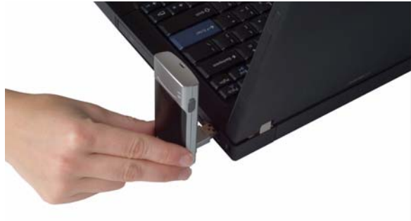
Figure 2-11: Correct way to insert the AirCard modem
