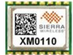
AirPrime™ XM0110 GPS module based on SiRFstarIV™
